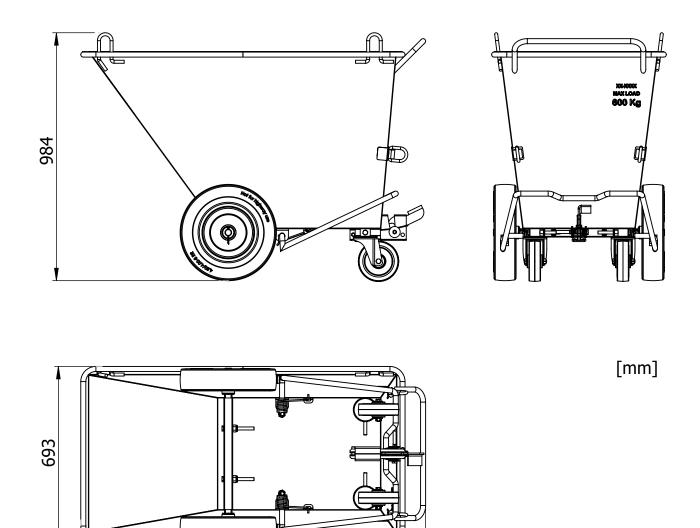
Volume: 355L Weight: 65 kg. Max load: 600kg.
